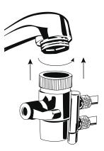
Make certain that gasket (already installed in diverter valve) is positioned securely between the diverter valve and the faucet (or adapter). Rotate diverter valve stem to desired positions. Swivel collar may need to be re-tightened. Place assembly conveniently next to sink.
