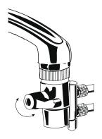
This causes the water to flow through the filter before exiting the faucet. To stop water flow to filter, rotate the lever back to turn water off.
