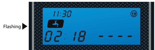
The display shows the Queued Regeneration in Meter Delay Mode.
